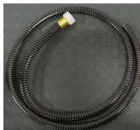
*Connecting brine discharge service hose at quick disconnect
