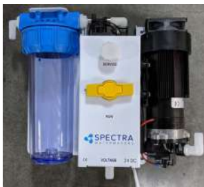
Service valve OFF, in FLUSH position
