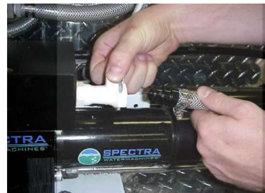
Connecting brine discharge hose:
